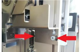
The lateral guards are both different from one another, one is for the left side and one is for the right side.
