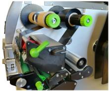
Once the foil is attached to the foil rewind wheel, rotate the rewind wheel until reaching the beginning of the ink strip and maintain the foil in tension.
