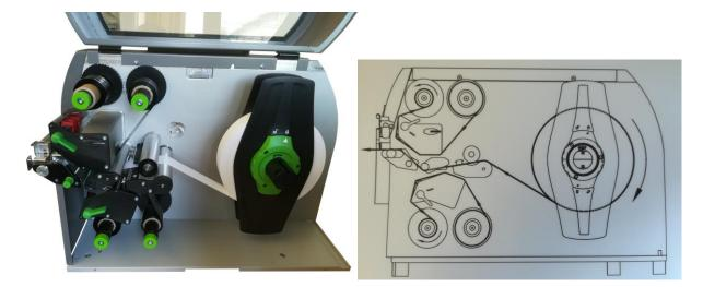
For ribbons with inner cores of 76 mm, it is necessary to use adapters for the supply holder (As shown in the images below).
