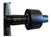
Once positioned, rotate the green locking ring on the extremity of the wheel counter-clockwise until the foil is locked in place.
