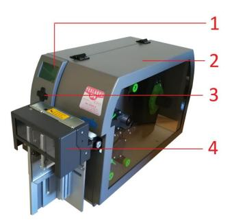
1. ON/OFF Switch and AC Power Port
