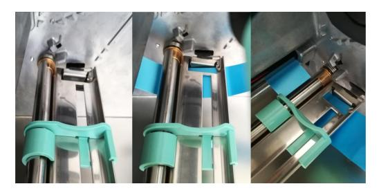
Pass ribbon through the printhead, making sure to also have the white arrow of the sensor (circled in red in the picture below) positioned above the ribbon being printed.
