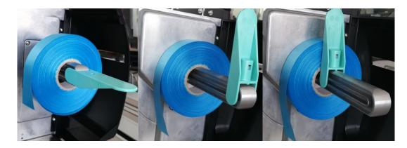
Pass the ribbon through the guides and adjust to width of ribbon.
