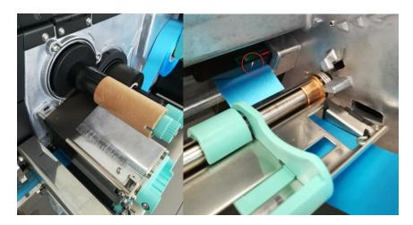
Lower the printhead latch by rotating it until it closes properly.
