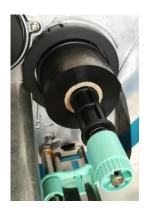
Insert empty cylinder core into foil rewind holder
